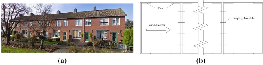
Fig. 1 a Typical Dutch terraced houses; b prescriptive rules for the design against wind load (NEN 2012)
