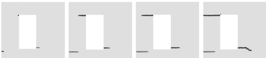
Fig. 15 Sequence of crack propagation for different steps in the repetitive test of TUD-Comp 41
