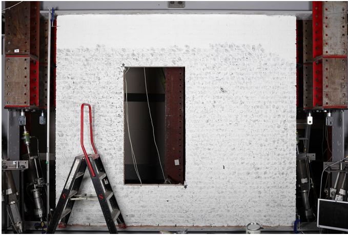
Fig. 5 Photograph of one of the experimental walls, before the application of the DIC pattern has been finished
