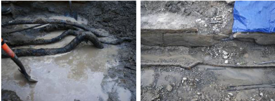
Fig. 2 Examples of typical curvature damage observed amongst buried cables due to the Canterbury earthquakes. Photos courtesy of Andrew Massie at the Christchurch Polytechnic Institute of Technology
