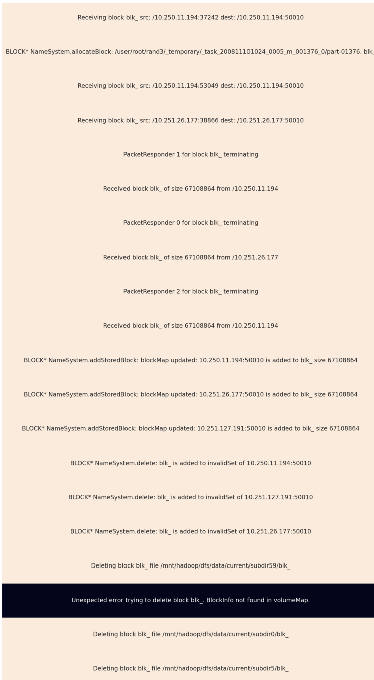
Fig. 6 Suspiciousness map of various anomalous samples from the HDFS dataset that were detected as anomalies by the model for the occurrence of a fatal event. Darker colors represent more suspicious events
