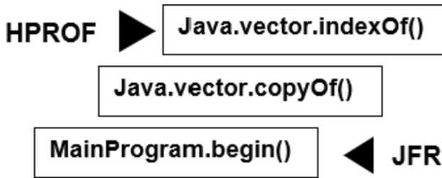
Fig. 1 Example of a call stack: three methods in a call stack showing the bottom of the stack, found by JFR and the top, found by HPROF. This is a fundamental difference in the way HPROF and JFR approach sampling. JFR will stop walking up the trace at the code that is part of the project being profiled ( MainProgram.begin() ) whereas HPROF will pick up the API function Java.vector.indexOf() . This API function is not editable; so we walk back up the trace to find the calling function MainProgram.begin() . In some cases, this trace back to the target project is not available. Figure taken from (Watkinson and Brownlee 2023)
