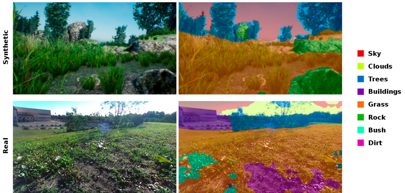
Fig. 4 Segmentation outputs of the employed DeepLabV2 backbone on synthetic and real image samples, demonstrating the high realism of synthetic images and the accuracy of the segmentation model
