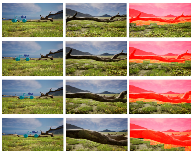
Fig. 11 Examples of traversability estimated when facing a horizontal obstacle in mid-air. Each row of images shows a side view of the scene, the agent's camera view and predicted traversability
