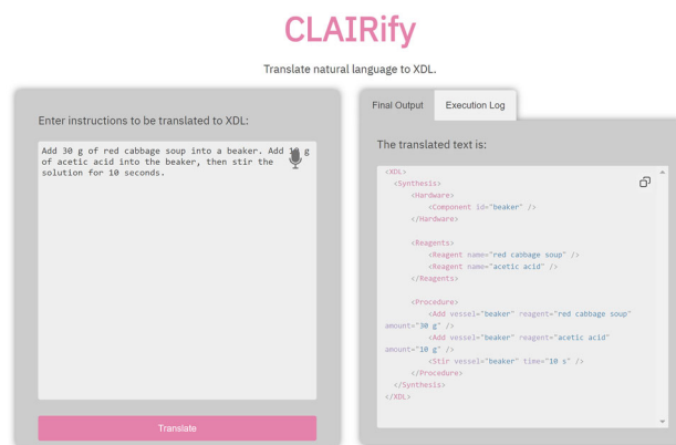
Fig. 4 Web interface for CLAIRIFY. Users input natural language descriptions of the experiment in the left column. XDL is generated in the right column when the user pushes the Translate button
