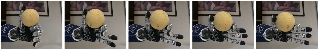
Fig. 1 Example regrasp trajectory generated by our method and executed using the iCub robot. The grasp posture changes from a lateral pinch to a tip pinch
