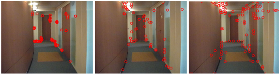
Fig. 3 Feature points found using: (left) ORB, 46; (center) SIFT, 61; and (right) SuperPoint, 87
