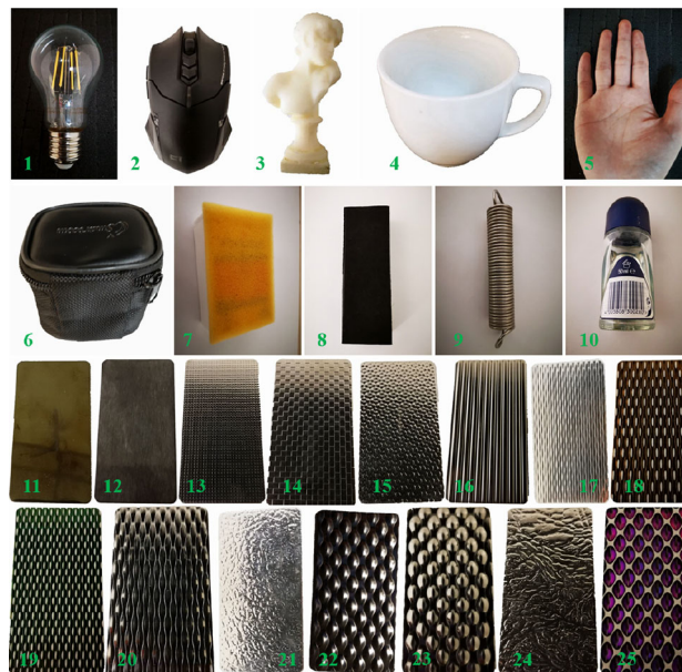
Fig. 9 The objects used in the haptic exploration experiments. From top to bottom, left to right is: bulb, mouse, 3D printed statue, cup, human finger, soft box, sponge (softer), black sponge, metal spring, glass bottle; and plates made with different materials and patterns: mirror stainless, satin stainless, BA stainless (canvas), BA stainless (squares), BA stainless (13SD), BA stainless (cambridge), BA stainless (11PS), bronze stainless (pippin), green stainless (poppy), BA stainless (5WL), BA stainless (2WL), BA stainless (7GM), BA stainless (6WL), BA stainless (9EH), red stainless (pearl)
