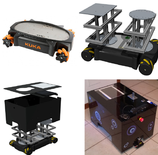
Fig. 2 Design process of KuBo. The overall height of the robot is about 30 cm and a new cover, made of black opal methacrylate, is mounted to an internal frame. The last picture shows the final prototype
