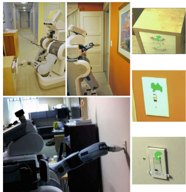
Fig. 1 Left Willow garage PR2 operating a drawer, light switch and rocker switch using learned detector that detects regions where manipulation will succeed. Right Results from learned detectors during execution
