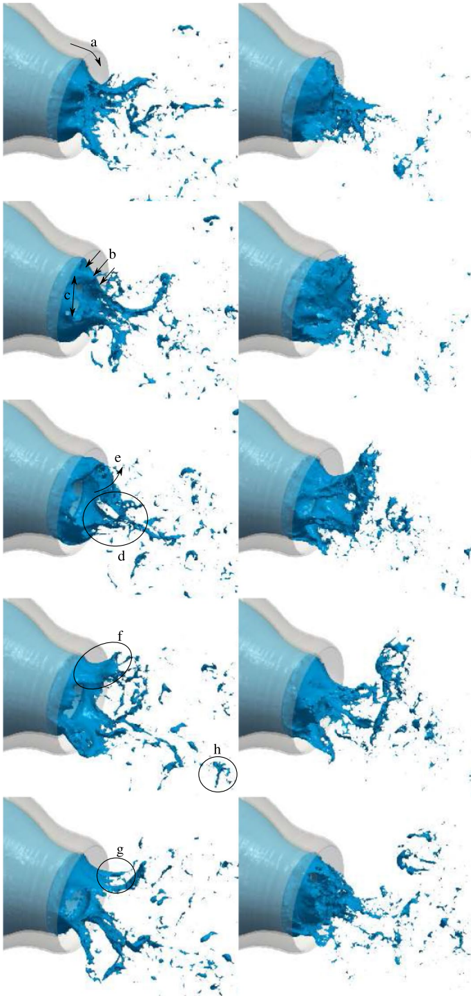
Fig. 11 Time series of a breakup event for L_1 (left, \Delta t = 71.6 \mu s ) and L_2 (right, \Delta t = 28.2 \mu s )
