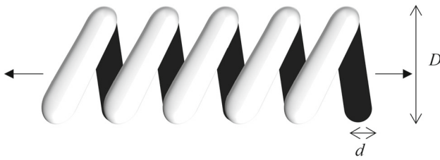
Fig. 7 A schematic diagram of a tension/compression spring design
