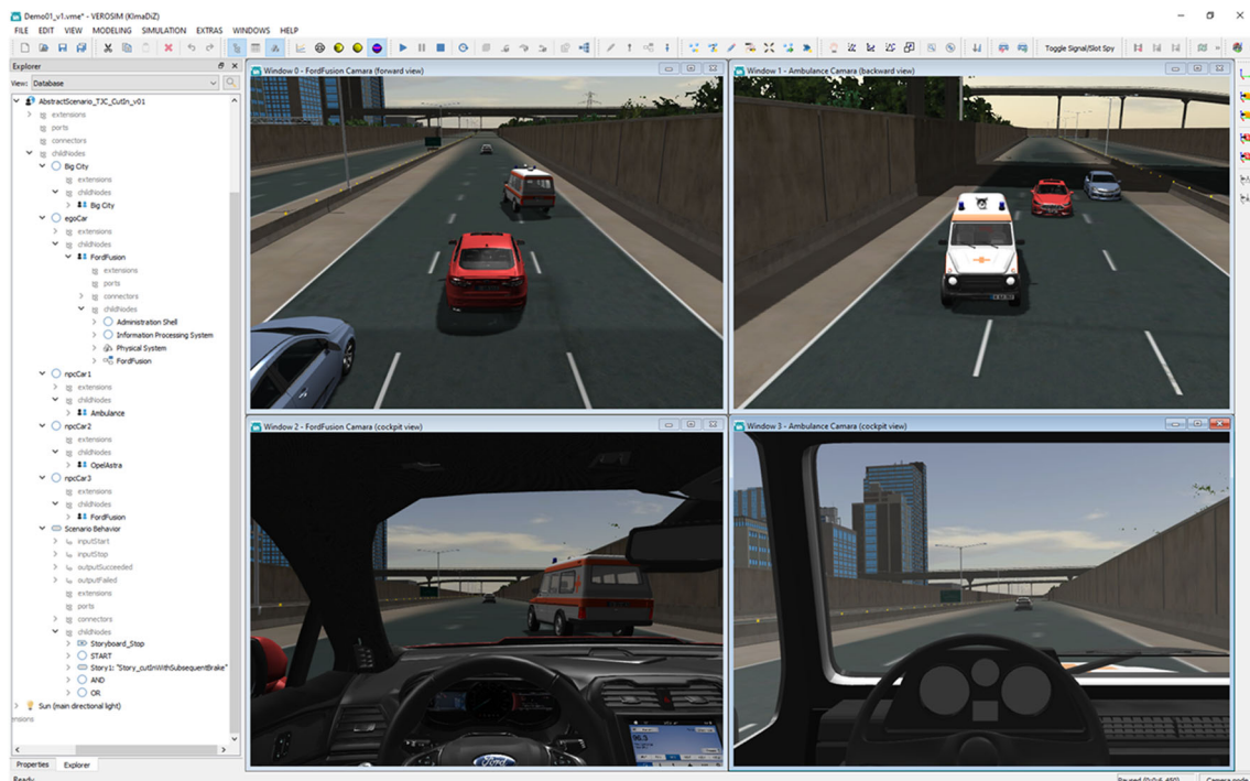
Fig. 6 Execution of the simulation scenario inside the virtual testbed showing different views on the cut-in process simultaneously
