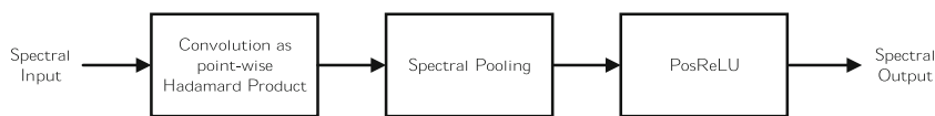
Fig. 2 Functional architecture of feature-extraction blocks for the SpCNN models used in this work
