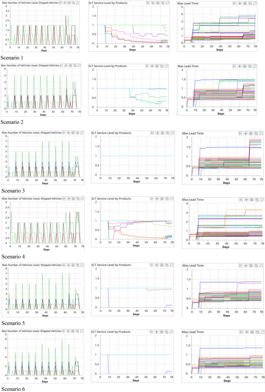
Fig. 12 Comparison of the vehicle usage, service level, and maximal lead time of the test scenarios
