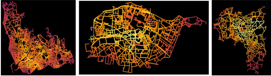
Fig. 6 Visualization of the three studied regions in terms of closeness centrality: (on the left) Matosinhos, (on the middle) Paranhos and (on the right) Maia
