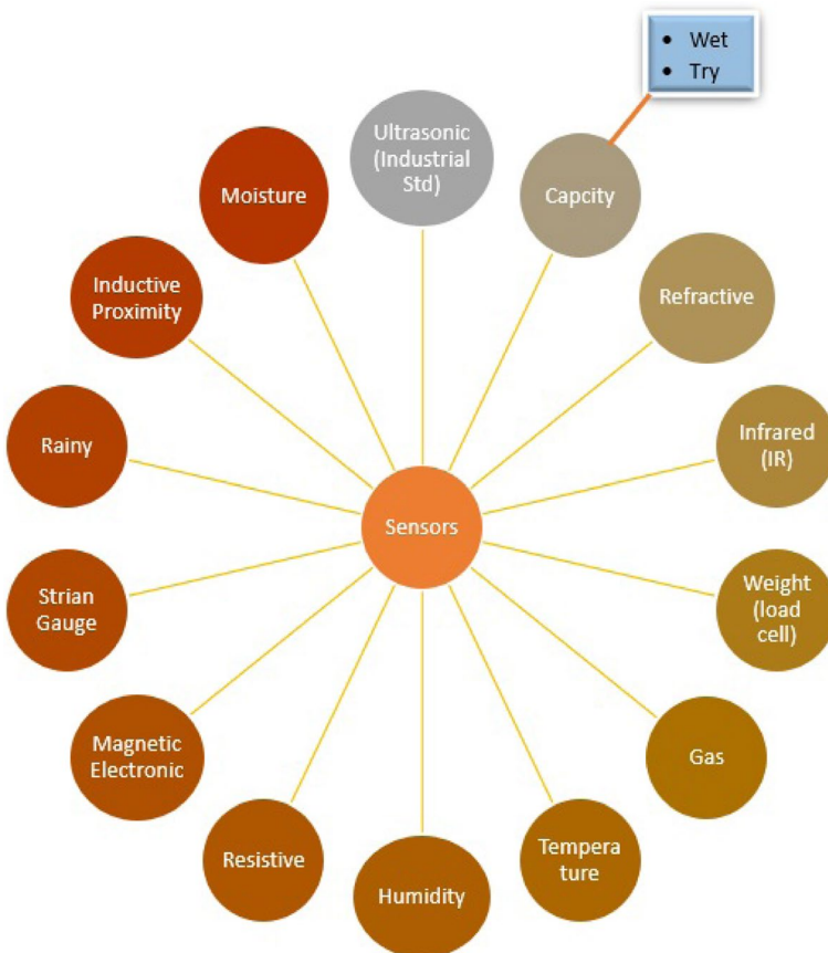
Fig. 7 Various sensors in smart bins
