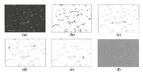
**Fig. 40** The processing of the actinomyces image. **a** Original image. **b** The binary image after a two-step thresholding. **c** The skeleton selection. **d** The whole skeleton with branches. **e** The whole pruned skeleton. **f** The triple points and end points on the skeletons (in Grivet et al. (1999) Fig. 3)
