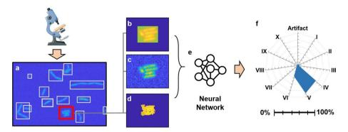
**Fig. 24** The work flow of image processing. **a** The image is binarized and annotated manually. **b** Null Bumper. **c** Blended. **d** Masked. **e** Neural network training. **f** The input of neural network (in Tamiev et al. (2020) Fig. 2)
