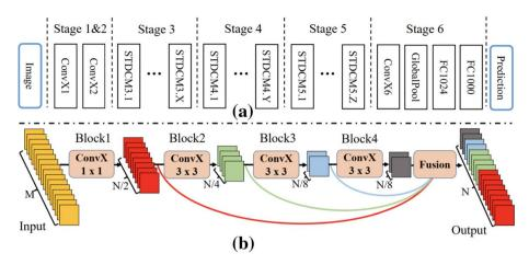
Fig. 53 a The original architecture of STDC network. b The proposed architecture of STDC network (In Fan et al. (2021) Fig. 3)
