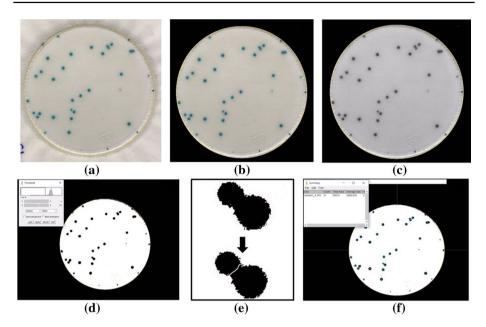
**Fig. 44** ImageJ automated cell analysis of a Petrifilm image. **a** Petrifilm colony forming area outlined with the oval ROI tool. **b** The area outside the ROI is cleared. **c** Image is converted to 8-bit. **d** Threshold is set to highlight colonies as black particles. **e** Merging colonies split by a single pixel line via the Watershed tool. **f** Particles included in the total count, highlighted and numbered in an overlay on the image (In Stolze et al. (2019) Fig. 1)
