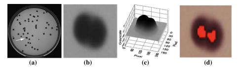
**Fig. 39** Detection of 2 overlapping colonies of E.coli. **a** 2D shadow image of agar plate. The arrow points to the cluster of overlapping colonies. **b** Magnified image. **c** 3D shadow image. **d** 2 colonies recognized in the cluster (in Ogawa et al. (2012) Fig. 6)
