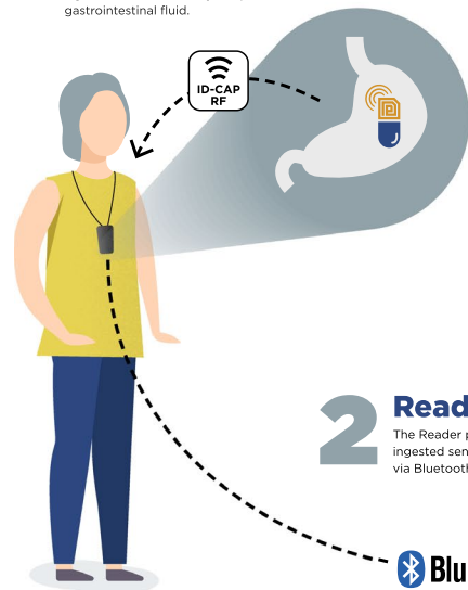
Fig. 1 Overview of digital pill system (DPS). The DPS includes an ingestible sensor within a gelatin capsule that over-encapsulates a medication. When ingested, it is activated by gastric fluid, broadcast-
