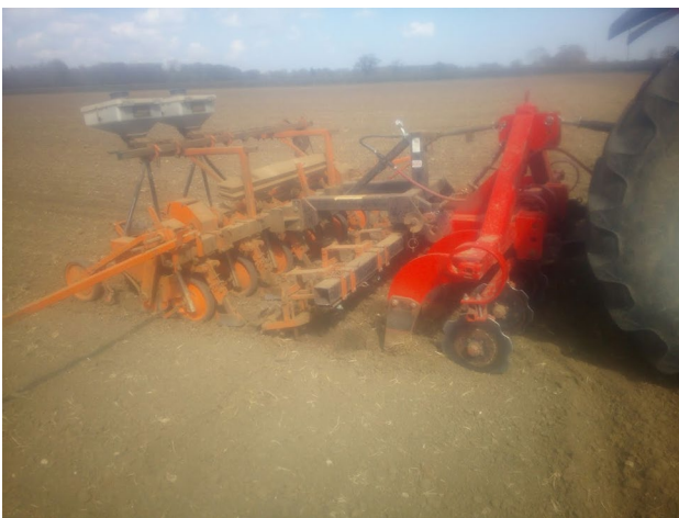
Fig. 7 Farmer invention: beet drill time bar. Farmer description: “The red bar started life in front of a potato planter, then was recycled to carry six compaction removing legs, with leading discs sourced from a drill breakers yard. The middle section (row crumbler) came from an auction, under which is a spray bar from a redundant sprayer, applying a biostimulant to promote better rooting. The tank on the front of the tractor was previously used 12 years ago with a sprayer we had at the time. The micro granule applicator on the back of the drill was used by a previous owner for nematicide and is now used to sow crimson clover seed between the beet rows to attract beneficial insects that eat the virus carrying aphids that infect sugar beet.”
