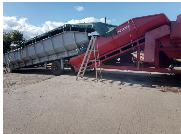
Fig. 5 Farmer invention: feed potato grader to hold potatoes. Farmer description: "The grey hopper holds 14tons of potatoes and was previously part of a carrot line in a supermarket packhouse. We built the chassis and fitted the axle that its now on to make it mobile and suitable to fit into our system. It starts and stops automatically via an ultrasonic sensor to feed the grader on demand, and its capacity has saved us a tractor, trailer and operator all season, worth today about £400/day. It cost £11,500 to build including the modifications
