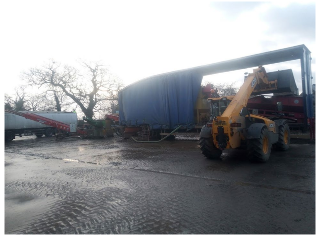
Fig. 8 Farmer invention: Mobile potato washer. Farmer description: “This is the biggest of our recent projects, a mobile potato washer. Most washers need a hopper and elevator to feed them, and so are static. We built one into a 45' curtain-sided step frame trailer. A second-hand donor grader provided a sensor-controlled hopper and coils and all of the cross conveyors. This is fed directly with the forklift, the coils remove any loose soil, then they go up a flighted elevator surplus from a redundant box filler on farm, into a 3×1 m barrel washer sourced from a redundant packhouse in Ireland. On exit they are rinsed onto a picking table and head out through the headboard of the trailer into another flighted elevator which feeds them into a remote-controlled telescopic elevator and into the lorry. The green section in the line is a destoner, which we put in the line for various customers, but not all. The pickers are protected from wind, rain and cold, and now have much more comfortable working conditions... Cost £42,000. Saving minimum £25,000/year.”
