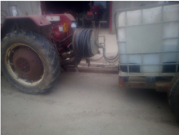
Fig. 6 Farmer invention: Water cart for drain jetter. Farmer description: “We used a scrap beet cleaner bridge axle to make a trolley to carry two 1000L ibc tanks to hold water to feed the drain jetter/power washer fitted on the tractor linkage. It didn't cost much and saves a lot of chasing about and hassle. Easy jobs get done, hassle stops them being done!”
