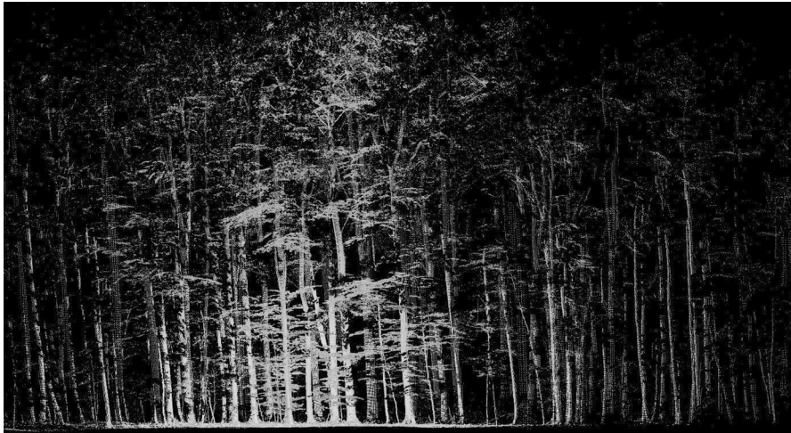
Fig. 3 2D representation of the 3D point cloud of an exemplary forest reference scene obtained from a single scan in leaf-less condition
