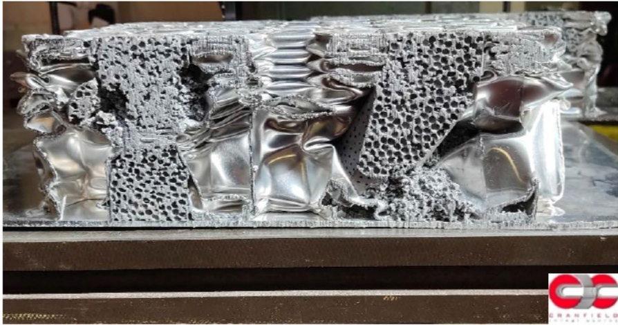
Fig. 20 Cross section of experimental results after impact test
