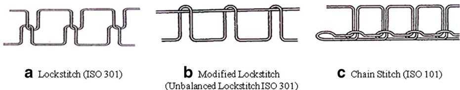
Fig. 1 Typical stitch types used for through-thickness reinforcement; (a) Lockstitch, (b) Modified Lockstitch, (c) Chain Stitch [11, 12]
