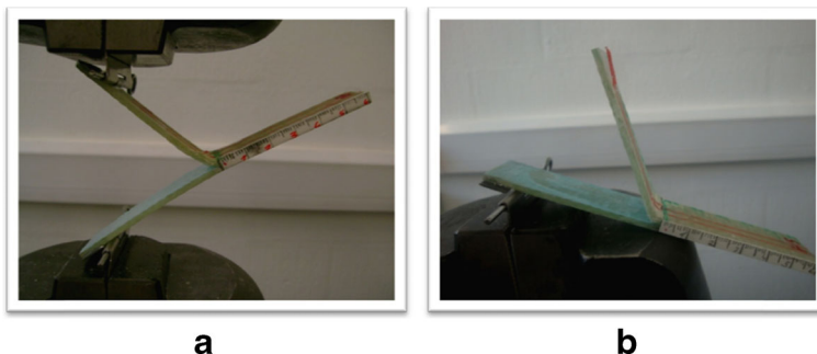
Fig. 2 a The top arm of the test specimen bent during the trial. b Detachment of metal hinge during testing
