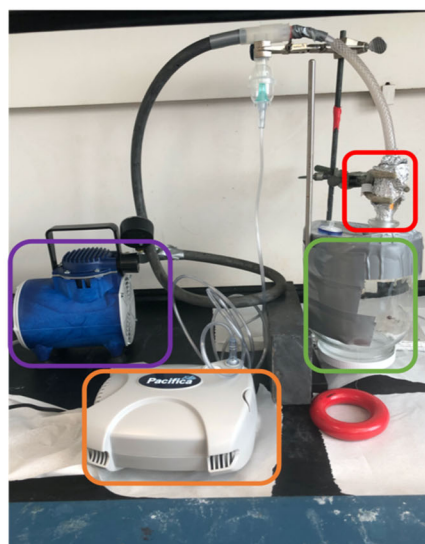
FIGURE 1. Experimental setup for modified PPE filtering and contact-killing efficiency in vitro . In future work, the petri dish can be replaced by an Andersen cascade impactor for more detailed particle flow-through data.
