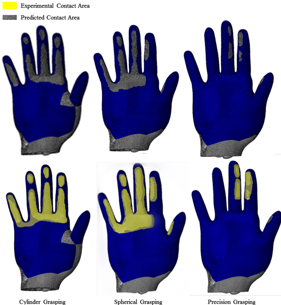
FIGURE 5. Comparison of contact area between experimental measurement and FE prediction.
