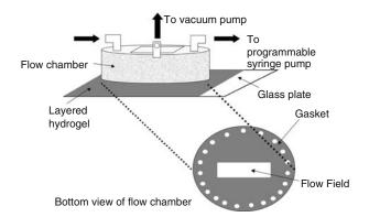
FIGURE 1. Schematic of parallel plate flow chamber system. A small pump is used to create a vacuum, sealing the chamber on the surface of the gel. Cells are then perfused over the gel surface using a programmable syringe pump.
