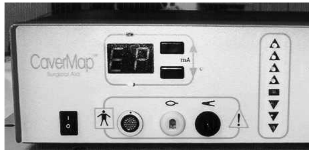
Figure 1. Control unit. The control unit contains the connectors for the probe handle and tumescence sensor. The unit displays the stimulation response with audible and visual signs.
