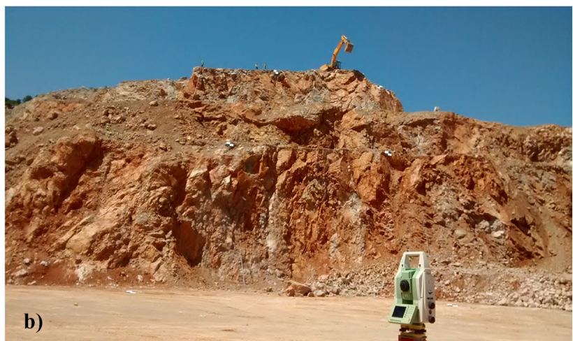
Fig. 5 General view of test 1 (a) and test 2 (b). Several blocks can be seen left and right of the bulldozer in (a). In (b) the total station is ready to position the black and white targets used as GCP, which are visible in the pictures
