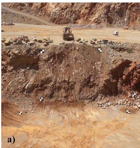
Fig. 5 General view of test 1 (a) and test 2 (b). Several blocks can be seen left and right of the bulldozer in (a). In (b) the total station is ready to position the black and white targets used as GCP, which are visible in the pictures
