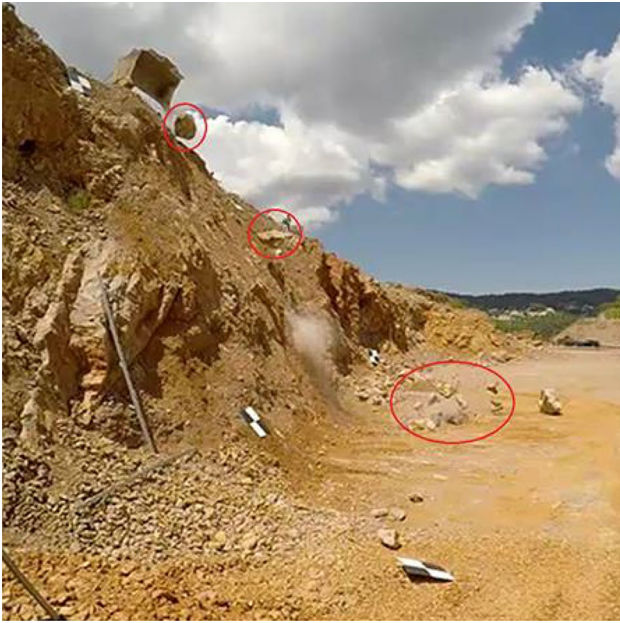
Fig. 8 Three frames (circled in red) extracted from a lateral shot, combined in a single picture at test 1. This block broke when hitting the lower esplanade
