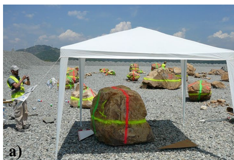
Fig. 3 Block conditioning before the drops, test 3 upper esplanade. Three major color “circles” were painted over each block surface. Then, a 360° photogrammetric survey was carried out (a). On the ground, left to the block, note the two red and white 1-m rods used
