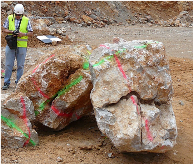
Fig. 16 Two limestone blocks that remained unbroken after the drop, although they exhibited some karstic dissolution features, partially cemented
