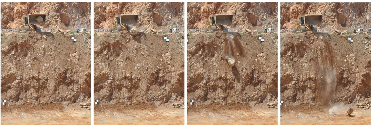
Fig. 7 Series with 4 frames extracted from a frontal view video at test 1. This block did not break, globally speaking, although some particles may have become detached from the corners
