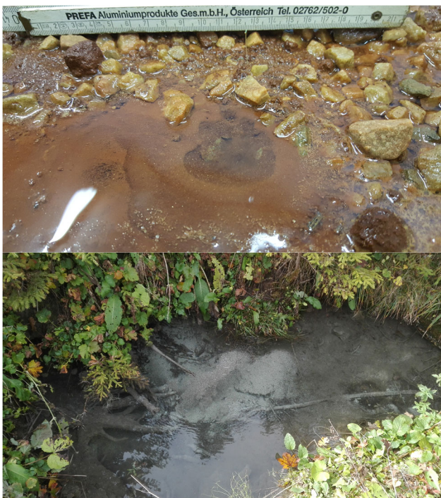
Fig. 12 Limnokrenes in the lab experiment and at the Fernpass near Biberwier. a Limnokrene developing during experiment no. 3 (electronic attachment 6). b Limnokrene near Biberwier (electronic attachment 7)
