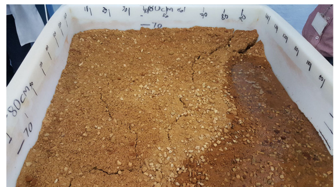
Fig. 10 Beginning of crack formation and a water-filled lateral depression during experiment number 1. Spacing of the marks 10 cm
