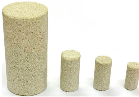
Fig. 1. Photograph of New Red Sandstone cylindrical rock samples used in the experimental studies, which sizes are listed in Table 1
