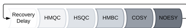
Fig. 12 Combination of five conventional, ^1\text{H} detecting nuclear magnetic resonance experiments into one time-saving supersequence that contains only one recovery delay. The sequence starts with a ^1\text{H} , ^{15}\text{N} HMQC (heteronuclear multiple quantum coherence) experiment as the most insensitive of all applied experiments, followed by more sensitive experiments, i.e., ^1\text{H} , ^{13}\text{C} HSQC (heteronuclear single quantum coherence), ^1\text{H} , ^{13}\text{C} HMBC (heteronuclear multiple bond correlation), ^1\text{H} , ^1\text{H} COSY (correlation spectroscopy) and ^1\text{H} , ^1\text{H} NOESY (nuclear Overhauser effect spectroscopy) experiments. The order of experiments from the least sensitive to the most sensitive is crucial to avoid disturbance between experiments. Figure adapted from Kupče and Claridge (2017)
