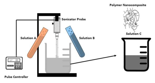
Fig. 6 Ultrasound cavitation technique in which a solution containing a nanopolymer composite is prepared after mixing two solutions A and B, and then a sonicator probe is immersed, and using a pulse controller, ultrasound is applied
