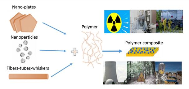
Fig. 9 Many forms of nanoplates, nanoparticles, fibers, tubes, and whiskers can be added to polymer matrix to synthesize polymer composites which can be used as radiation shielding materials in radiation facilities, nuclear power plants, and also nuclear cleaning of environment
