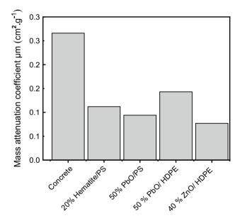
**Fig. 11** Mass attenuation coefficient of polymer nanocomposites: 20% hematite/polystyrene, 50% lead oxide/polystyrene, 50% lead oxide/high-density polyethylene, and 40% zinc oxide/high-density polyethylene compared to concrete
