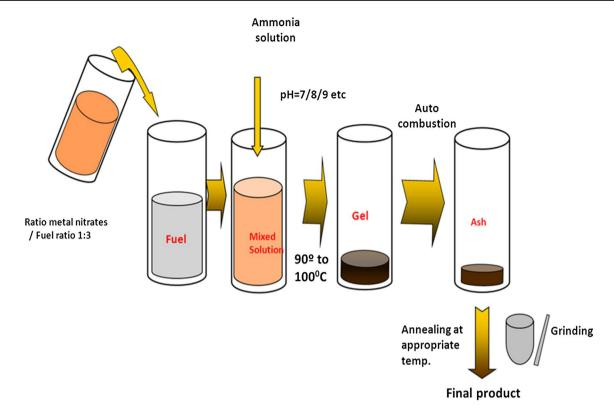
Fig. 5 Sol-gel synthesis of where a compound which contains a highly reactive component is solidified via sol-gel or solution which is followed by annealing and heat treatment
