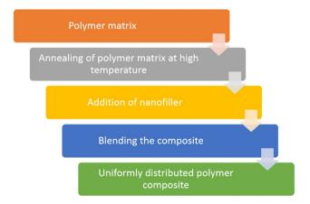
**Fig. 4** Melt intercalation method steps: preparing the polymer matrix which is followed by annealing at high temperature and then adding the nanofiller, and all the mixture is blended to form a uniformly distributed polymer composite
