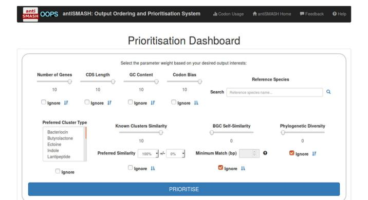
Fig. 1 OOPS graphical user interface. The weighing of each prioritisation parameter can be adjusted using the slide bar, or ignored by checking the associated box. The sorting order (ascending or descending) is specified by clicking the blue arrow icon. The refer-
