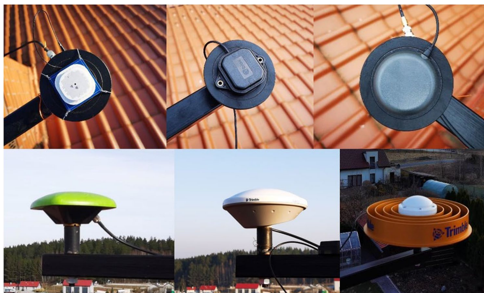
Fig. 1 GNSS antennas used in the experiment. The top row shows low-cost antennas ELT0149 (left), U-blox ANN-MB-00 (middle), and Tallysman TW7972 (right). High-grade antennas are given in the bottom row: JAVGRANT-G3T (left), TRM105000.10 (middle), and TRM159900.00 (right)
