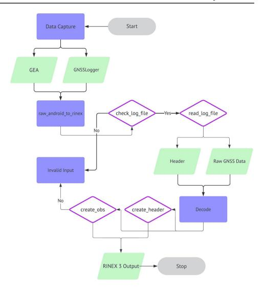
format, aligning with the structure proposed by the GNS-SLogger app. This standardized data input format ensures seamless compatibility, simplifying the conversion process and streamlining the utilization of raw GNSS data within the designated tool. For more details, please refer to Sect. 4.3 in the attached user manual of the tool.
