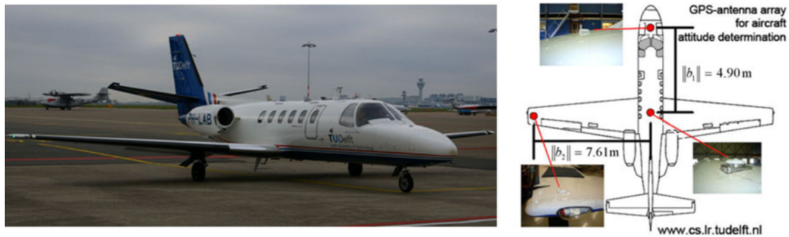
Fig. 7 The aircraft with antennae configuration
