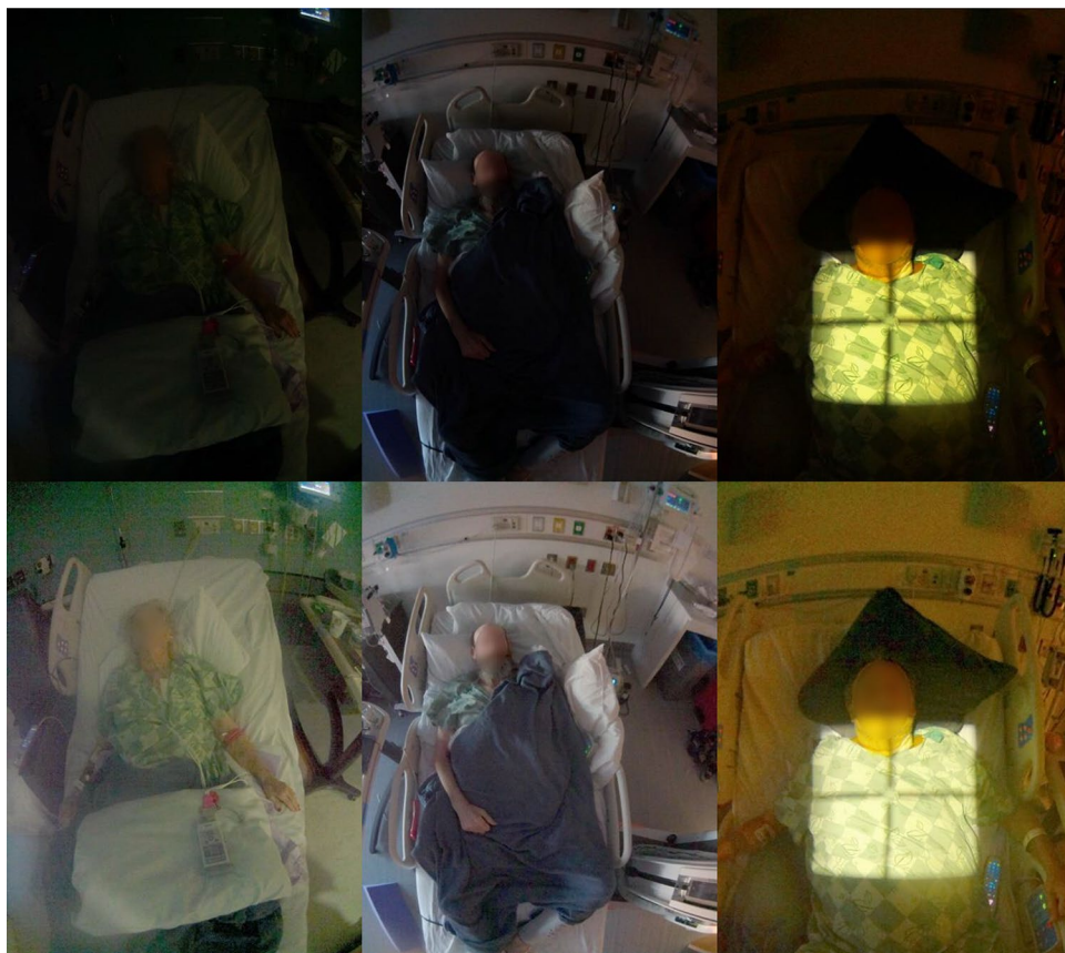
Fig. 7 Examples of automated gamma correction to reveal dark image regions. Original images are above, and corresponding, corrected images are below. Patient faces are blurred for privacy in publication but not in practice
