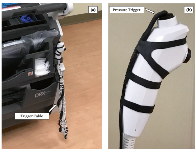
Fig. 3 a Initial hardware implementation for simultaneous triggering of photography acquisition. The pressure sensor is attached to the portable radiography machine trigger. b The camera trigger cable is strung along the radiography trigger cable showing how this can be tangled
