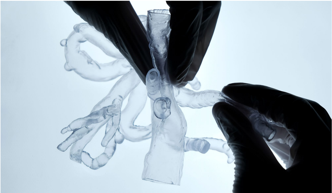
Fig. 3 Proof of flexibility and transparency of a CT-derived vascular model, printed with flexible resin. The aorta and its branches are easily compressed with two fingers, demonstrating the flexible quality of
