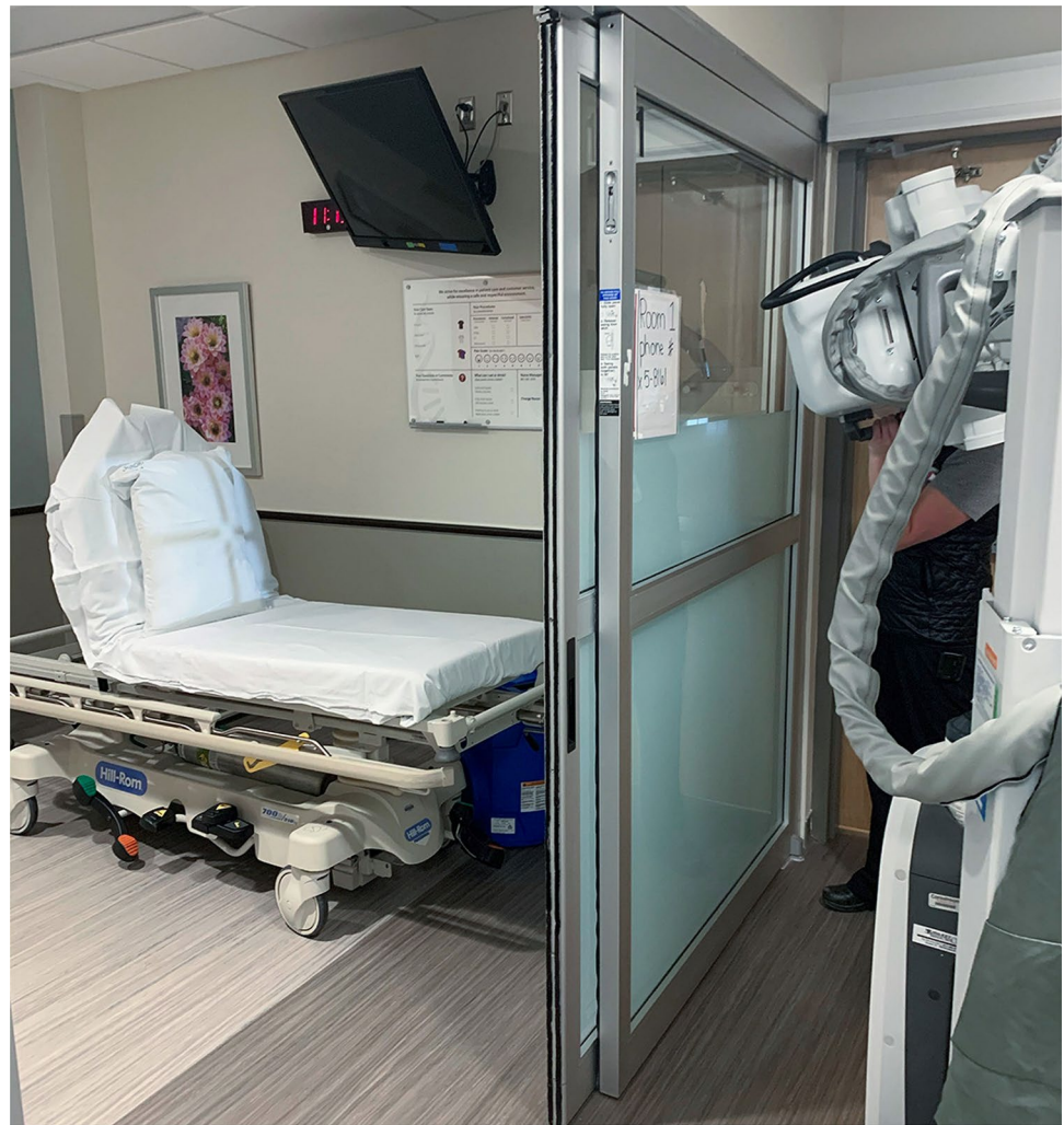
Fig. 1 Portable X-ray configuration at UHSB used to protect X-ray technologists taking care of patients under investigation for COVID-19
