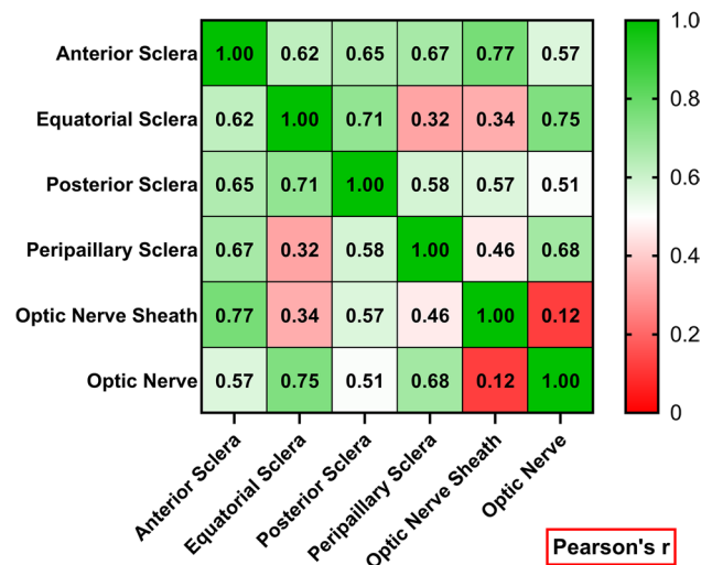
Fig. 8 Regional cross-correlation of tangent modulus among six ocular tissue regions at 3% strain
