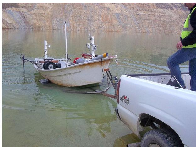
Fig. 3 Photograph of the remotely controlled boat used to sample and profile the Berkeley Pit
