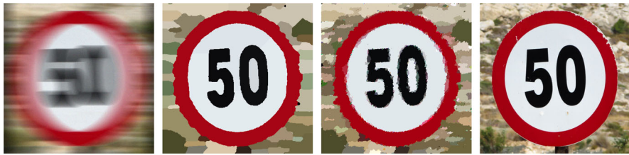
(a) Blurred and noisy data (b) Proposed, \gamma = 0.15 (c) Ambrosio-Tortorelli, \alpha = 10^5, \gamma = 0.8, \epsilon = 1/2 (d) Original
