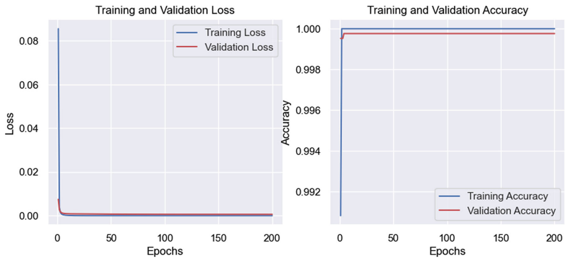
Fig. 6 Plot showing training and validation loss (left) and the training and validation accuracies (right) for MQTT-IoT-IDS2020 dataset
