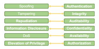
Fig. 2 Correspondence between the threat categories in the STRIDE model (left) and the security features (right)
