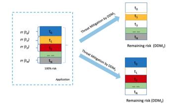
**Fig. 4** Functionality of module III. On the left side, we see the input of module III, the identified threats of an application with corresponding *risk ratios*. On the right side, we see the remaining risk of each threat after applying security countermeasures by the DDMs. White areas indicate zero risk, coloured areas indicate the remaining risk
