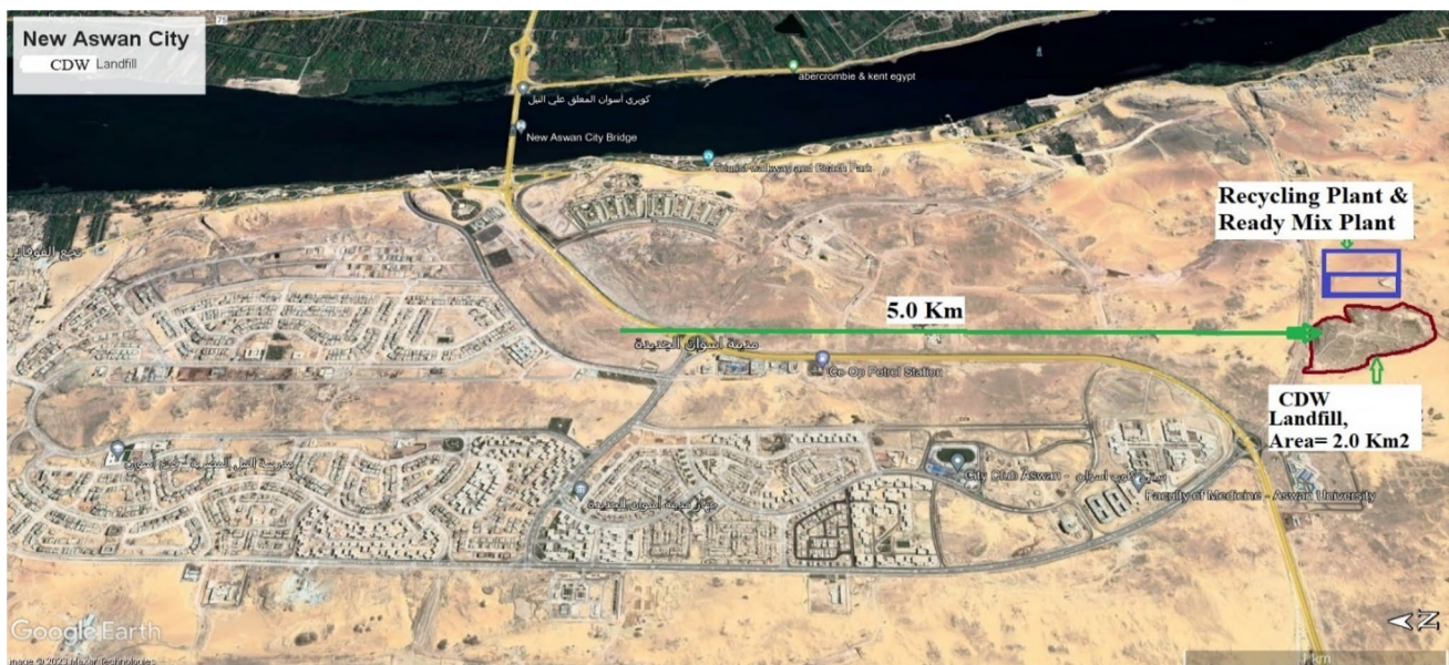
Fig. 3 The case study, including landfill, recycling plant, and ready-mix plant data
