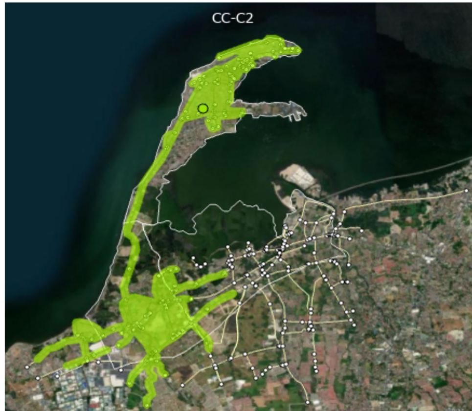
Fig. 5 15-min service area of CC-C2. The location of one of the selected temporary storage sites in Cavite City is represented by the circle and the areas it could serve by the shaded regions. Within 15 min, considering the assumptions, the site could serve portions of adjacent towns
