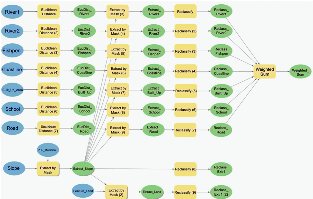
Fig. 2 Temporary storage siting model generated. ModelBuilder in ArcGIS Pro was used to create a series of procedures to generate results
