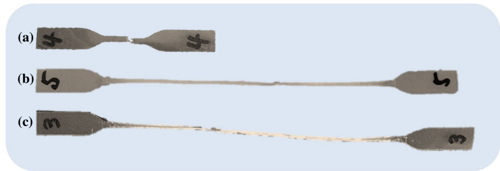
(a) Pre-RPP 210°C 2min SC, (b) Pre-RPP 230°C 10min Q, (c) Pre-RPP 250°C 10min Q
