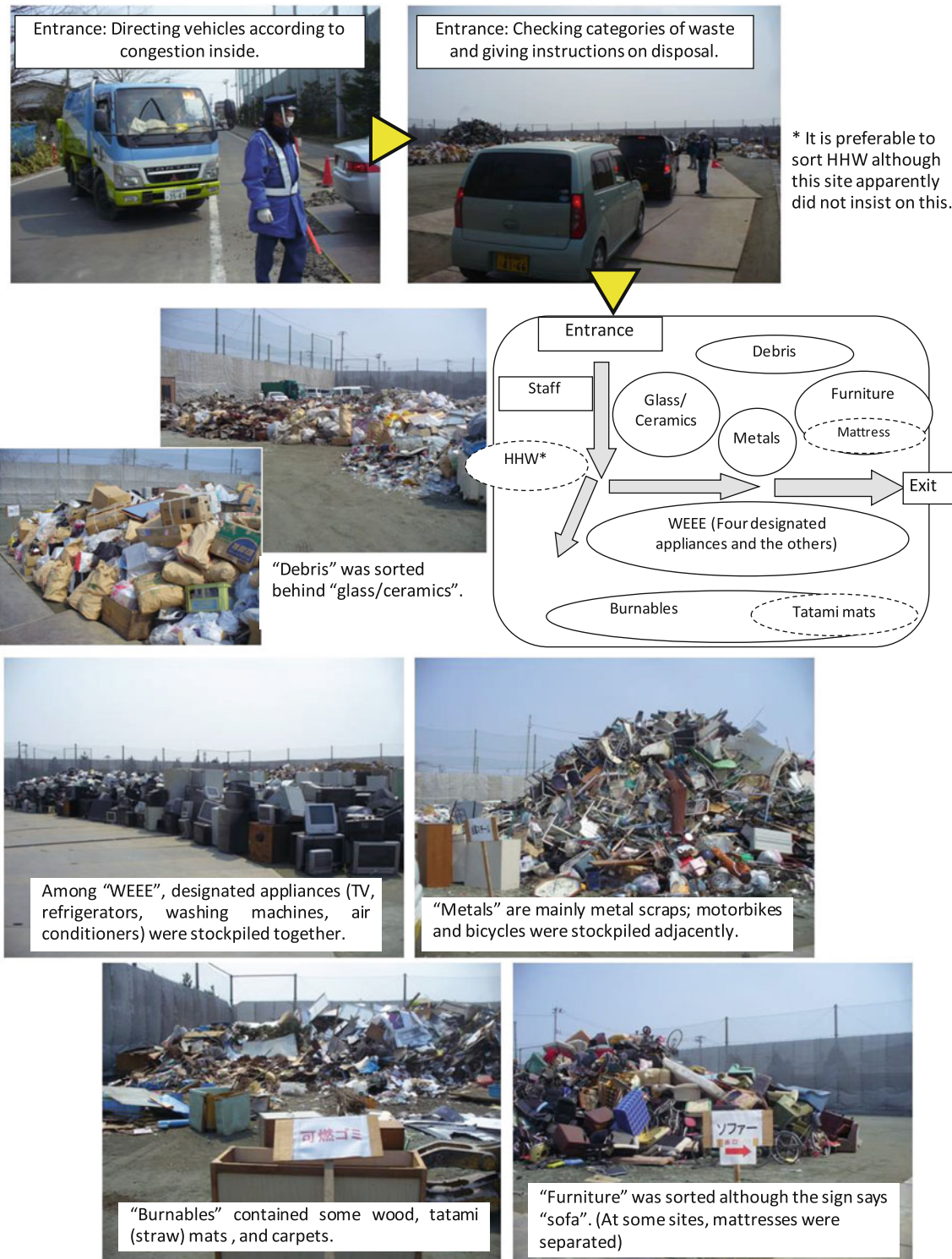
Fig. 2 Reference: A good example of management at a deposit (temporary storage) site for early recovery phase, Nipperia playground, Sendai city; workers direct and instruct how to sort and
